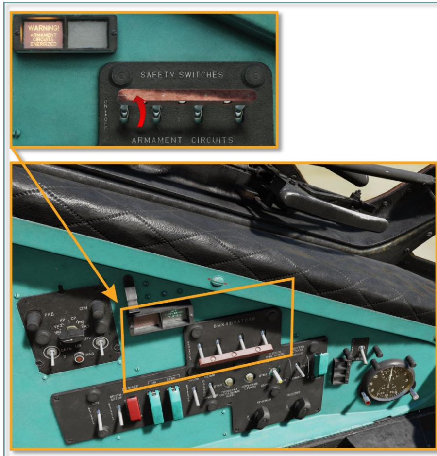
Fig. 4.12. Safety switches and signaling boards of their state
