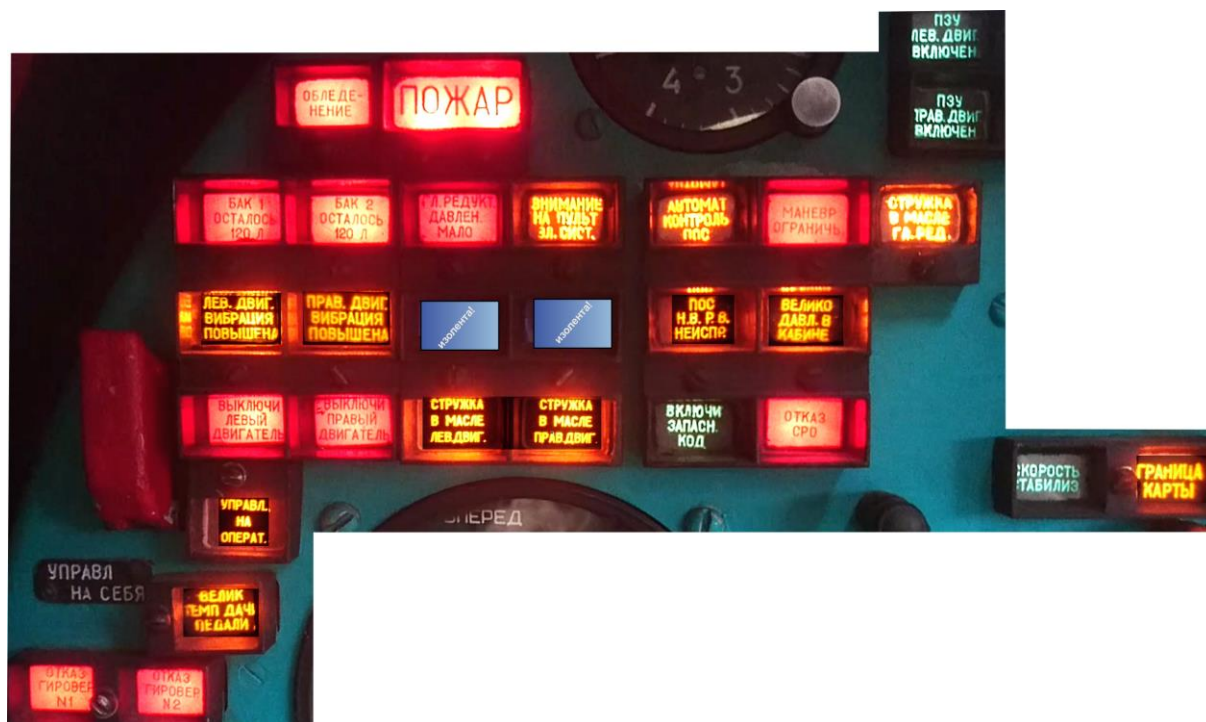
Fig. 1.7. Block of signal boards on the pilot's dashboard
