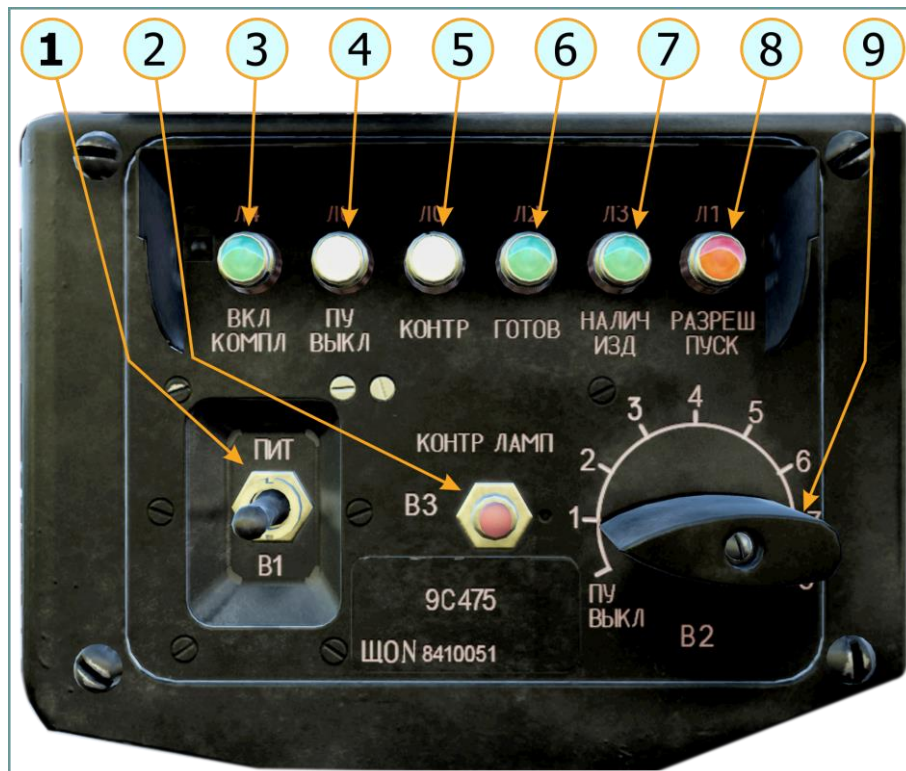
Fig. 4.16. Operator's panel (SCHO) (Power on-off and selection missile panel)
