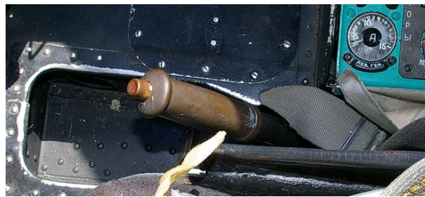
Fig. 1.14. Main rotor brake lever
