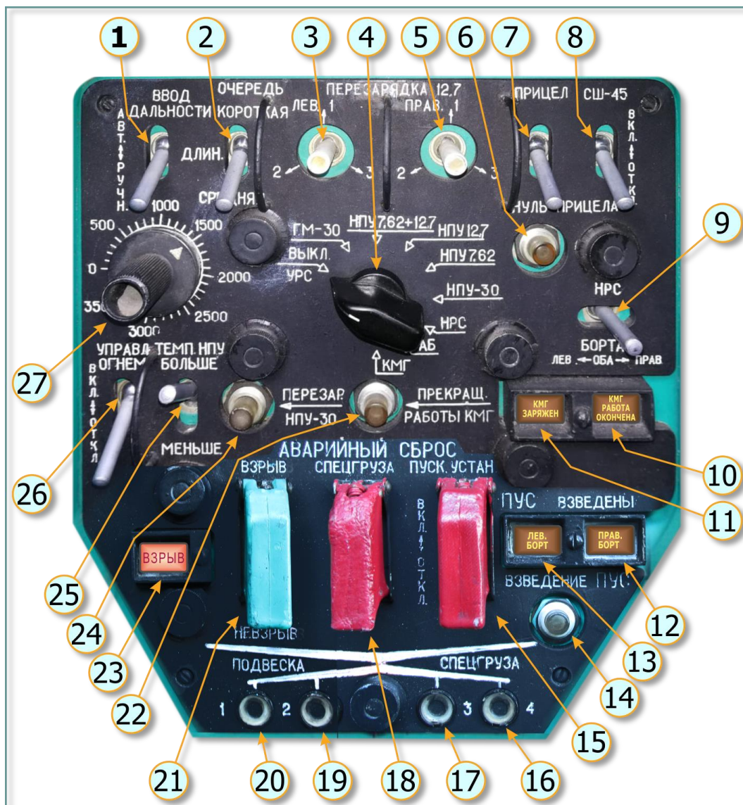
Fig. 4.9. Pilot armament control panel (PUVL)
